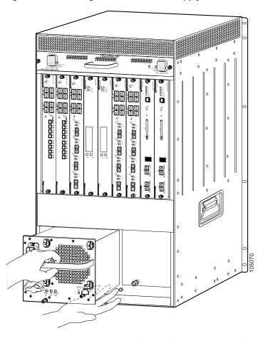
Figure 8 Installing the 3000 W Power Supply
